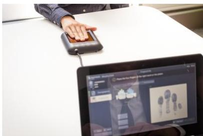
Based on the TFT (Thin-Film Transistor) technology, this new ultra-thin terminal allows the capture of 10 fingers flat or rolled. Its speed and quality of acquisition are incomparable (capture of the fingers possible in less than two seconds, improved performance for dry fingers, specific finish to avoid traces).
