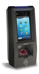
The terminal's high performance results from its ARM® Cortex™-A9 core powerful processor running best-in-class fingerprint algorithms - and its FBI PIV IQS approved biometric sensor.
