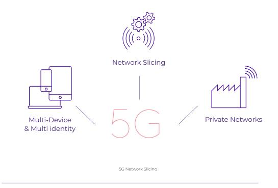
**5G network slicing** is a network architecture that allows for easy virtualization that is tailored according to business needs. Each network slice is an isolated end-to-end network designed to meet a variety of needs, such as those expressed by mobile operators, MVNOs, and enterprises.
